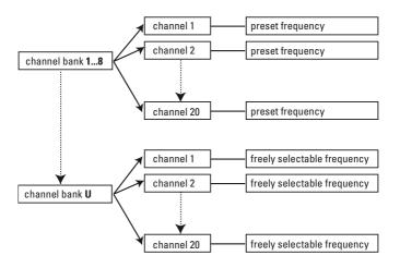
Each of the channels in the channel banks "1" to "8" has been factory-preset to a receiving frequency (see enclosed frequency table). These receiving frequencies cannot be changed but have been preset so that e.g. country-specific regulations on frequency usage are taken into account. The channel bank "U" (user bank) allows you to store your selection out of 1440 receiving frequencies that are freely
